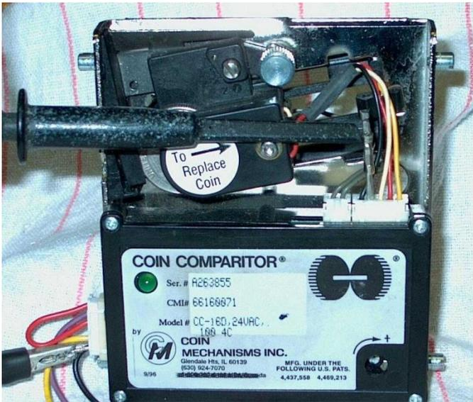
**Connect scope test probe to the "Test Point" J2 pin 4**
